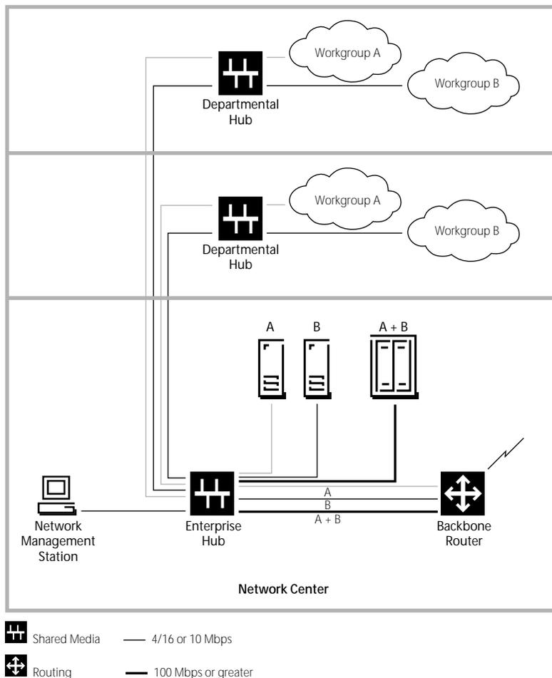
Enterprise hubs and network management also enable servers, even though centralized, to be coupled to their clients on the same segment with minimal latency. Centralized, high-capacity routers provide firewalling and wide area links, as well as intersegment communications. Server centralization greatly facilitates such functions as backup and software updates, thus reducing the overall cost of administration.
